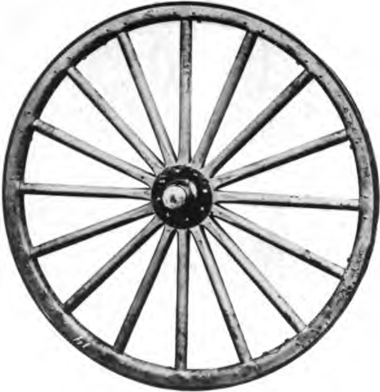
3-INCH FIELD CARRIAGE WHEEL. 16 SPOKES.
